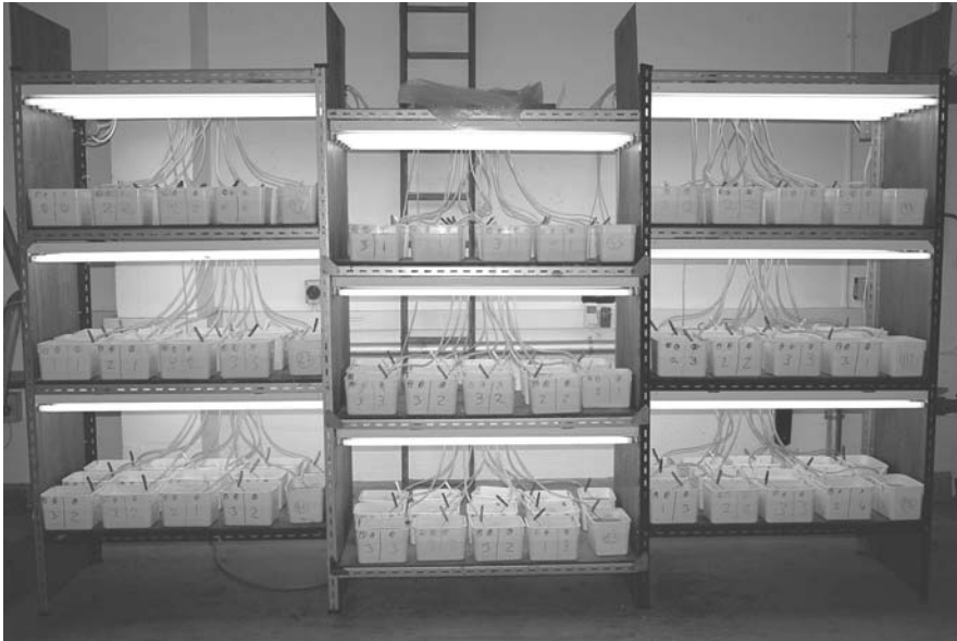
Fig. 4.6 Photograph showing the experimental set up. One nutrient is measured per container
